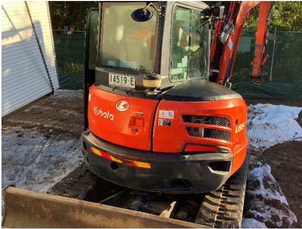
Photo 1: Excavator following decontamination of blade, buckets and tracks.
