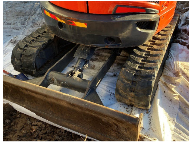
Photo 2: Excavator following decontamination of blade, buckets and tracks.
