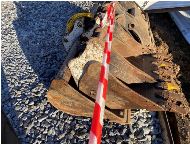
Photo 3: Excavator following decontamination of blade, buckets and tracks.
