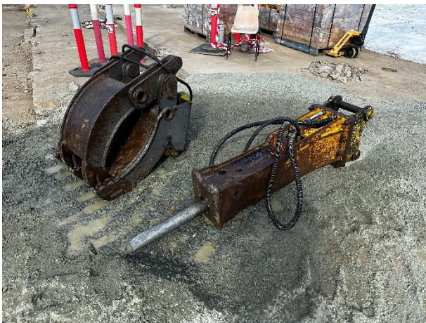
Photo 5: Excavator buckets and other attachments following cleaning.
