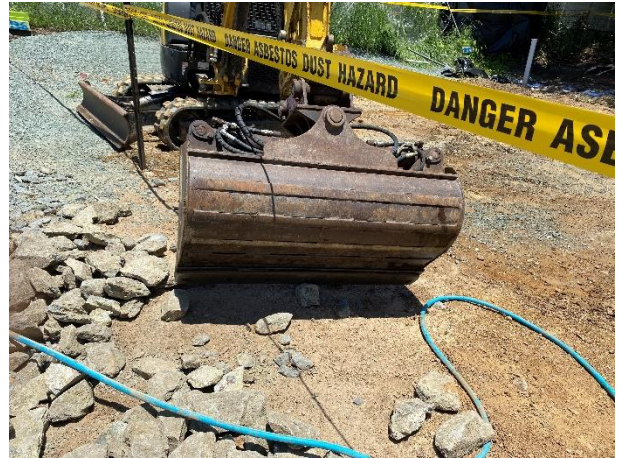
Photo 2: Excavator bucket following cleaning.
