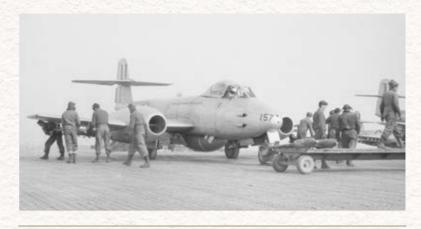
Ground crew of No. 77 Squadron RAAF arming a Meteor Mk 8 aircraft with high-explosive rockets for an attack on ground targets in North Korea. AWM JK0599
